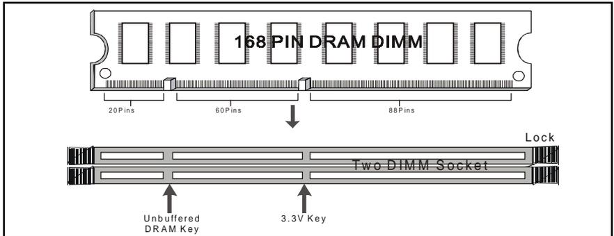
168-Pin SDRAM Module Installation Diagram
