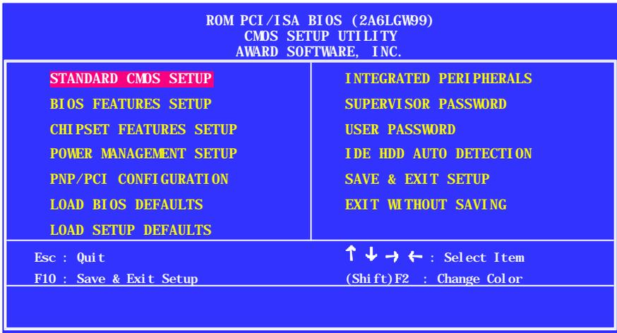
3. Using the arrows **↑↓→←** on your keyboard, select an option, and press **<Enter>**. Modify the system parameters to reflect the options installed in your system. Otherwise you may return to the Main Menu anytime by pressing **<ESC>** .
